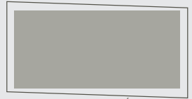
POOR BASE POSITIONING (CORNERS NOT AT RIGHT ANGLES)
